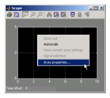
**5** In the Scope window, point to the *y*-axis shown in the figure below, and right-click.
