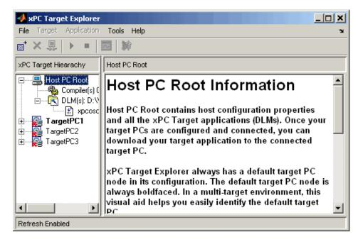
**5** In the xPC Target Explorer, expand a target PC node.
