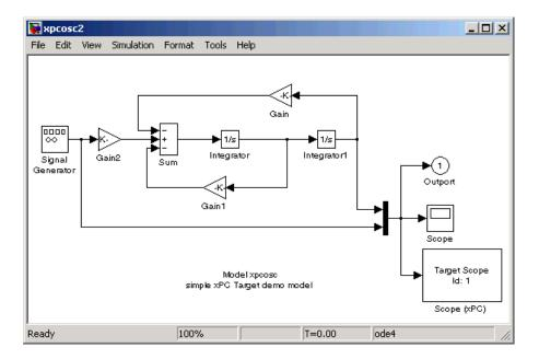
**4** To rebuild the target application, in the Simulink window and from the **Tools** menu, select **Code Generation**. From the code generation submenu, click **Build Model**.
