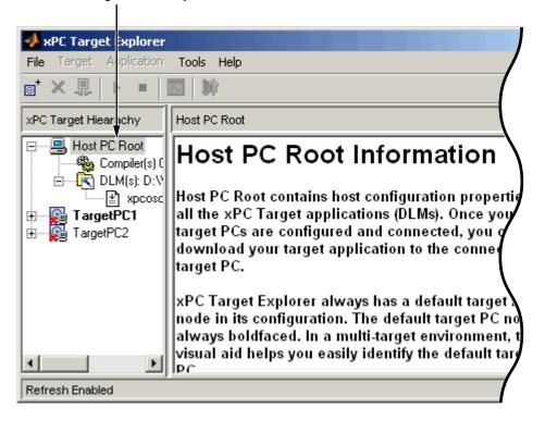
You can also start xPC Target Explorer from the Simulink model window (Tools > Code Generation > xPC Target Explorer).
